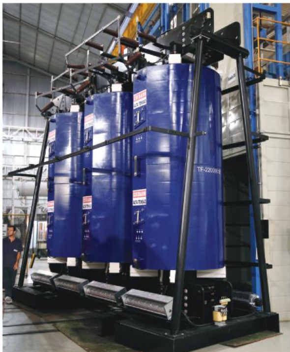
Fornecimento: PETROBRÁS 31,5MVA 36/15kV
